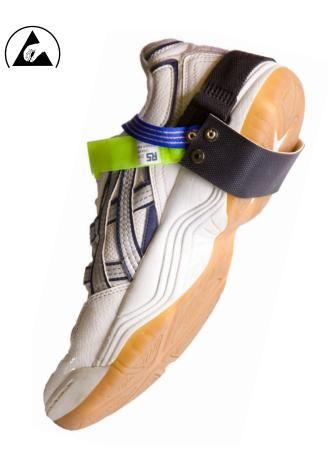
The heel grounder is constructed using a 36mm wide strip of two-layered rubber sheet with an insulative white and a conductive black layer attached to a 25mm wide elasticated back forming a heel cup. The heelgrounder has a 1 megohm resistor joined in series with the conductive tab. It is assembled with a separate hook and loop tape for adjustment.
