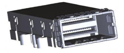
Specifications: Mating force : 210N min. Unmating force : 42N min. Durability : 250 cycles Max. PCB insertion force : 25N per pin Current rating : 0.5 amps max. per pin
