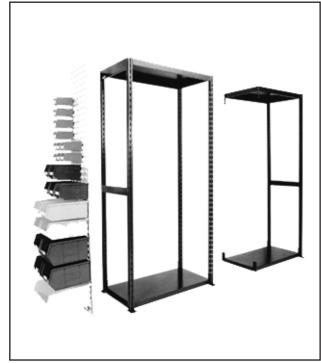
The basic and additional bays shown above must not have a combined UDL (uniformly distributed load) that exceeds 945kg. Therefore each bay must not exceed 945kg and the shelves must not individually exceed 135kg UDL.
