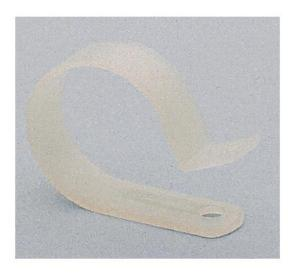
Material: UL approved Nylon 66, 94V-2 KSS CABLE CLAMPS are designed to hold cable, tubes, and components in domestic appliance, electronics and electric apparatus generally. Interior edges are radiused to protect cable insulation.
