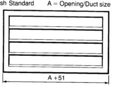
Louvres are manufactured in one piece units up to 1800mm square.
