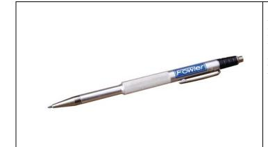
Pen Type scriber with pocket clip Retractable tungsten carbide point Aluminium and steel body with knurled grip Length 115mm, diameter 10mm, weight 40 gms. Supplied in a plastic wallet
