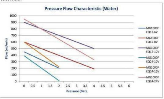
Pressure shown is the not to exceed value. All MG1000 pump variants are capable of more than the indicated figure but exceeding this may result in damage to the pump.
