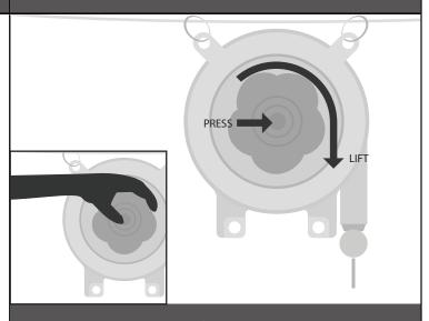
4. Press the rotator cover of the balancer with your thumb and lift up the rotator with your index and middle fingers. Turing clockwise will release the cord whereas turning counter-clockwise will fasten the cord.
