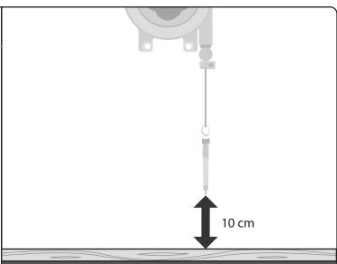
2. Loosen the screw of the steady ear first and adjust the distance between the screwdriver and the fastened item to about 10 cm.
