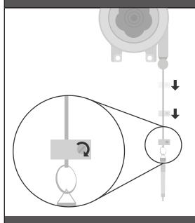
3. Move the steady ear towards the mouth of the balancer and fasten the screw.
