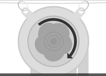
5. You can adjust the tensile level of the balancer by turning the rotator before use to avoid elastic fatigue which is caused by overload.
