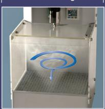
A powerful dust collecting fan exhausts dust quickly, preventing re-adhesion of dust.
