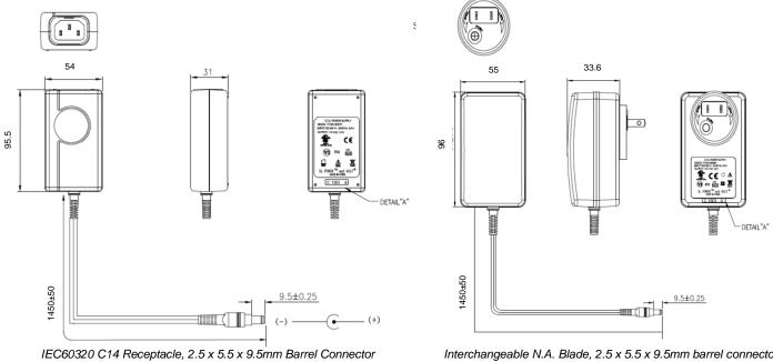
Notes: 1. All dimensions in mm. Interchangeable N.A. Blade, 2.5 x 5.5 x 9.5mm barrel connector
