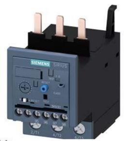
OVERLOAD RELAY 20...80 A FOR MOTOR PROTECTION SIZE S2, CLASS 10E FOR MOUNTING ONTO CONTACTORS MAIN CIRCUIT: SCREW TERMINAL AUX. CIRCUIT: SCREW TERMINAL MANUAL-AUTOMATIC-RESET
