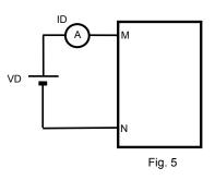
Switching time (The circuit is a representative example of the lower side U phase.)
