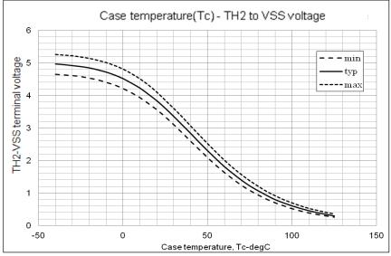
\*Condition : Pull-up resistor (RTH) =  $39k\Omega$  +/-1%, Pull-up voltage of VTH= 5V +/-0.3V Refer to application circuit.
