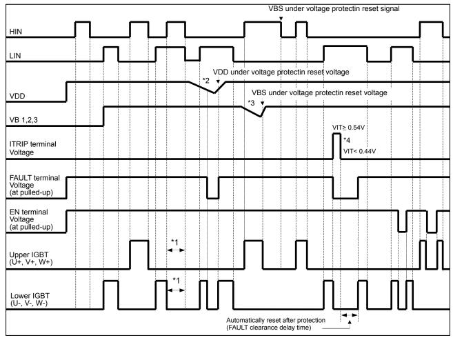
After the V<sub>DD</sub> turned on, the HIN voltage do not pass the IC until LIN voltage come.
