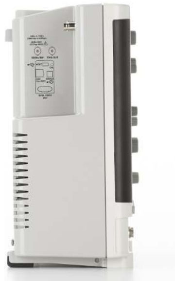
Figure 8. One-gigahertz-per-inch form factor: 6 GHz, 6 inches deep.
