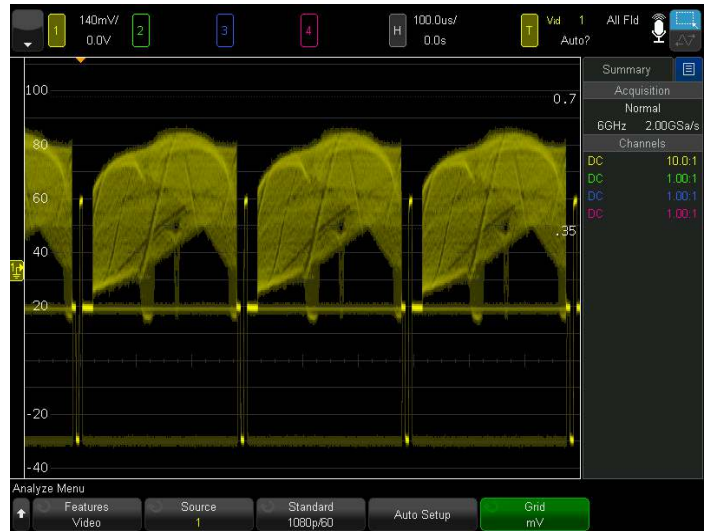
Figure 45. Triggering on a 1080p/60 signal.
