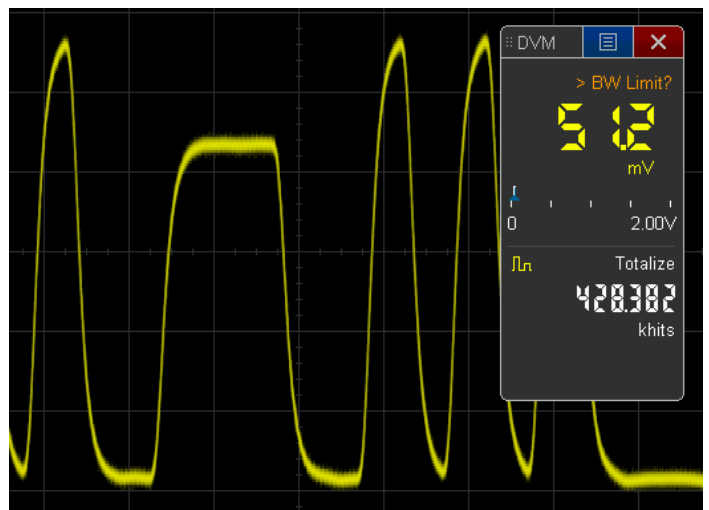
Figure 35. Totalizing the number of runt errors.
