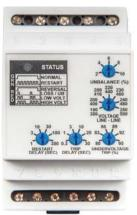
The Voltage Line-Line knob on the PMDU has two ranges (left): a 190-250V low voltage scale and a 380-500V high voltage scale. The unit auto senses the three-phase line-line voltage when applied and automatically selects the appropriate range.
