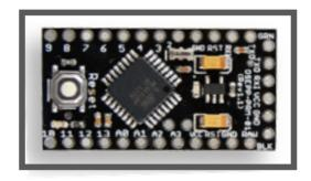
The OSEPP Pro Mini board is a miniaturized version of the OSEPP Pro, which in turn is a stripped down version of the OSEPP Uno. Basically, this is as small as it gets which allows for easy concealment in projects.
