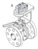
Finally perform a mechanical check of the assembly and a functional check of the position feedback.
