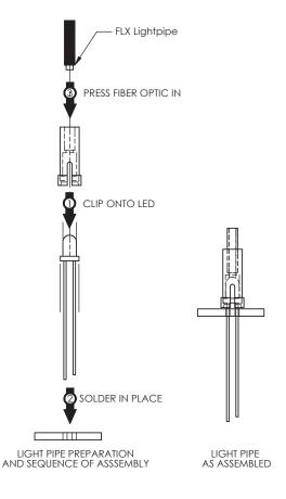
These LED couplers are suitable for use with VCC FLX series flexible lightpipe assemblies, resulting in a highly efficient coupling between LED and lightpipe.
