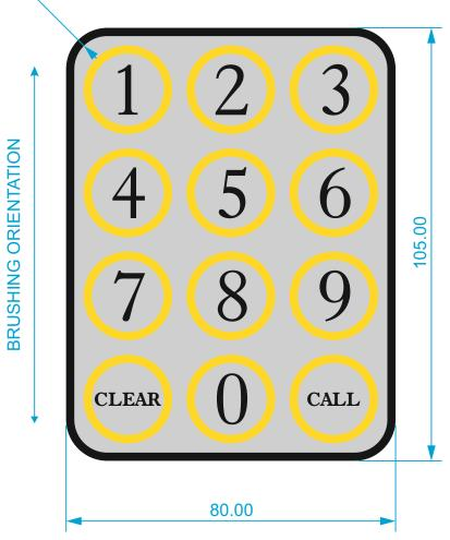
Material to be \$150 with brushing. Key pad to have 19.5mm dia. black circles around 12 tactile keys with 1.0mm printed UV perimeter emboss.
