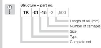
This order example (TK-01-15-2, 500) corresponds to a complete DryLin<sup>®</sup> system of size 15 with 2 carriages and 500 mm rail length.
