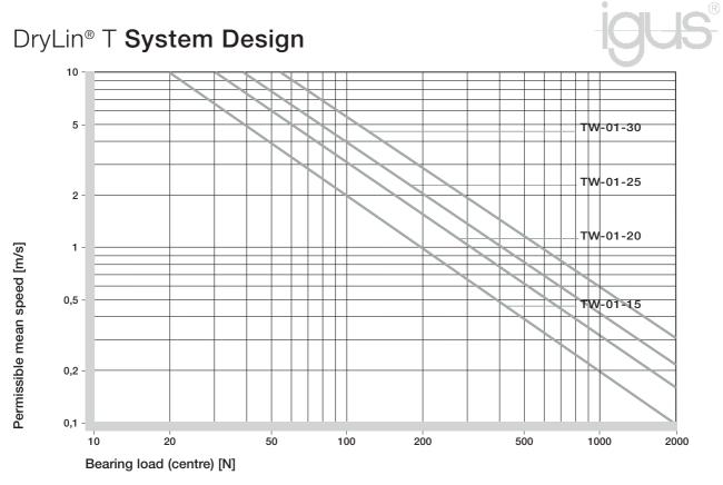
Graph 61.3: Graph to determine the maximum permissible speed for the calculated bearing load
