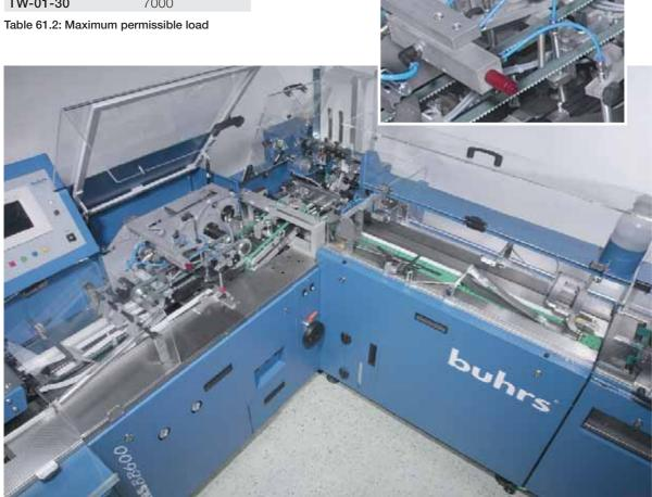
DryLin® T linear guide systems are used in these enveloping machines to guide a suction opener for envelopes. The guide system must have low clearance, be maintenance-free and not require any lubrication.
