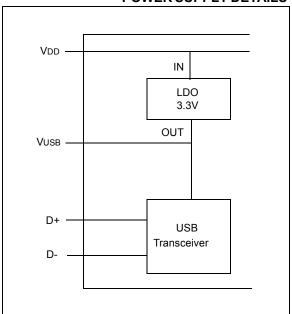
The provided VDD voltage has a direct influence on the voltage levels present on the GPIO and UART Tx/Rx pins. When VDD is 5V, all of these pins will have a logical '1' around 5V with the variations specified in Section 4.1 "DC Characteristics".
