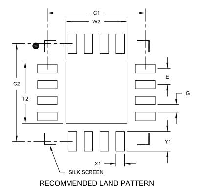
Units MILLIMETERS **Dimension Limits** MIN NOM MAX Contact Pitch 0.65 BSC Ε Optional Center Pad Width W2 2.50 Optional Center Pad Length T2 2.50 Contact Pad Spacing C1 4.00 Contact Pad Spacing C2 4.00 Contact Pad Width (X16) X1 0.35 Contact Pad Length (X16) Y1 0.80 Distance Between Pads G 0.30
