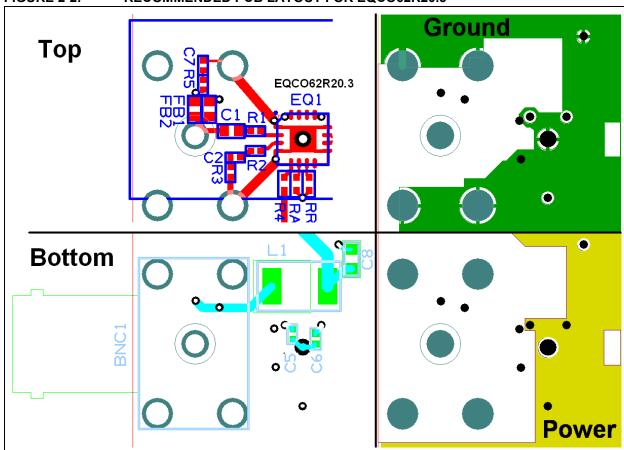
In this layout, the size of the PCB area needed for the chip is minimized. Approximately two times the BNC footprint area is required for the full bidirectional system: including the necessary elements for the power transport.
