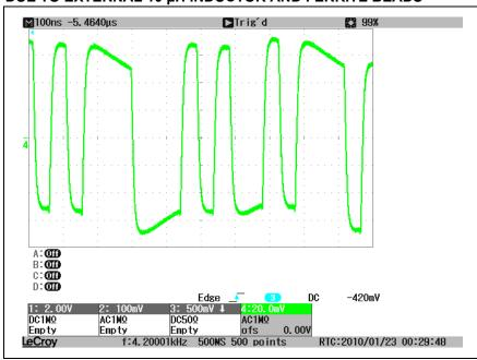
1: Inductor and ferrite beads at the camera side of the link will double the baseline wandering. This is resolved by the LF-Receiver in the EQCO62T20 chip.
