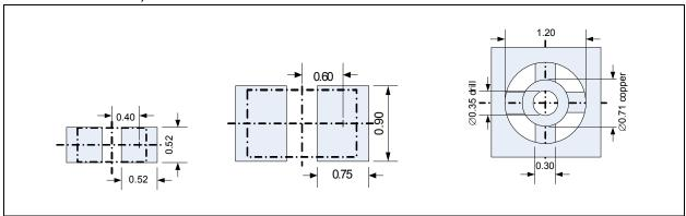
FIGURE E-2: DIN1.0/2.3 AND L1 INDUCTOR 1812 FOOTPRINTS
