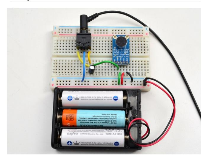
Connect the amplifier, battery pack and headphone jack as shown above.
