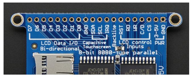
Make sure you're soldering and connecting to the 8-bit side!
