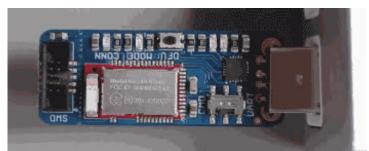
Using your favorite terminal emulator (http://adafru.it/iCU), connect to the BLEFriend at **9600 baud** with HW flow control enabled.
