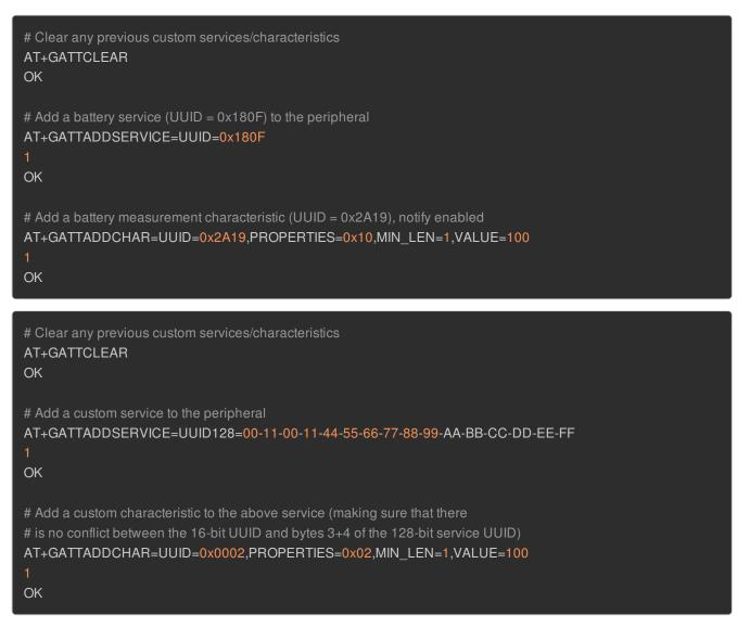
Version **0.6.6** of the Bluefruit LE firmware added the ability to use a new '**UUID128**' flag to add custom 128-bit UUIDs that aren't related to the parent service UUID (which is used when passing the 16-bit '**UUID**' flag).
