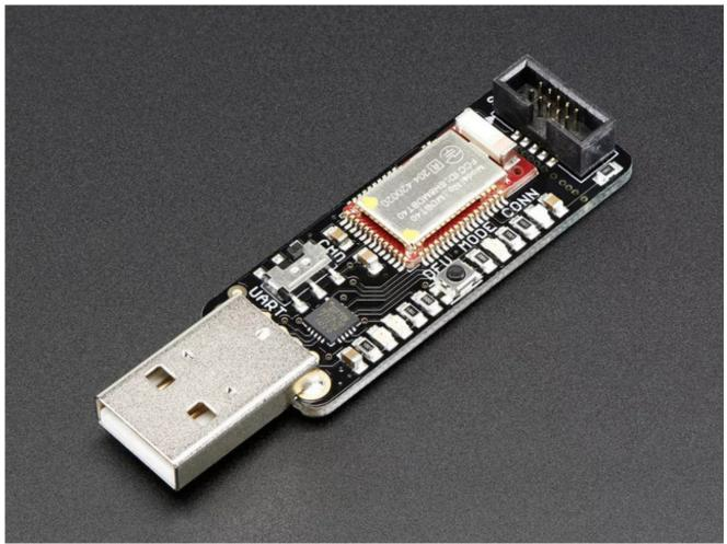
In it's simplest form, it works on the same principle as a common USB/Serial adapter (the FTDI Friend (http://adafru.it/dQa), for example!). Any data that you enter via your favorite terminal emulator on your development machine will be transferred over the air to the connected phone or tablet, and vice versa.
