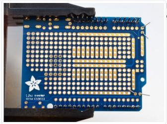
Bend the two little capacitor leads out so that you can flip over the PCB without the caps falling out
