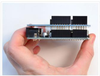
spare Arduino. Make sure all of the long pins plug into the sockets on the side of the Arduino. There will be a gap between the shield and Arduino and the Printed Circuit Board will be loose
