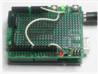
If you want to use the red and green LEDs or the general purpose button, simply solder solid-gauge wire (~22awg is good) into the large solder holes near the device. Then you can plug the other end of the wire like a jumper into any of the female headers. The two LEDs are tied to ground through 1K or 1.5K resistors. The button simply connects the jumper to ground when pressed (use an internal or external pull-up). Check the schematic on the download page for specific details.
