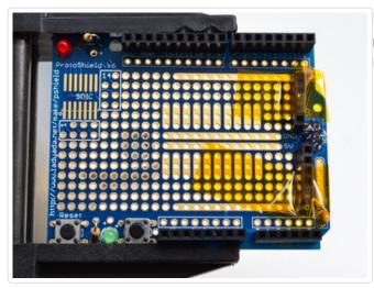
Place the two non-stacking 5-pin headers into the matching slots on the right hand side of the PCB. Use tape to keep them in place
