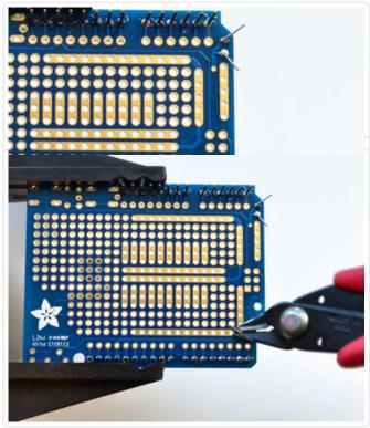
Then clip the leads short using a pair of diagonal cutters
