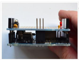
Plug the shield on top so that the 6 pins go through the matching holes in the PCB
