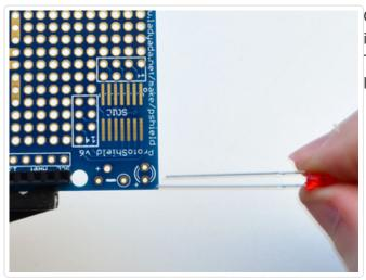
On the Proto Shield PCB, you'll see a circle indicating where the LED goes, and a small + sign. That's the indicator for which pad gets the longer leg of the LED
