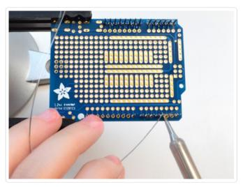
When done, check your work, make sure each pin is soldered with a nice shiny solder connection
