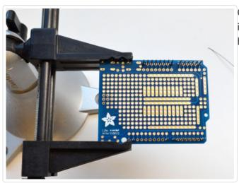
Carefully remove the shield from the Arduino and insert into your vise with the ends of the stacking header pointing up
