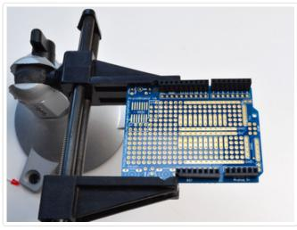
Start by placing the shield in a holder as shown, you shouldn't see the large Adafruit logo (its on the bottom)
