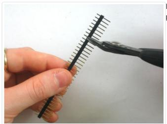
long strip. use diagonal cutters or pliers to clip off 4 parts, one 6-pin, two 8-pin, and one 10-pin
