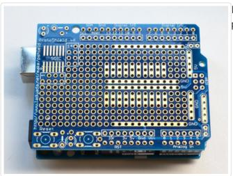
Place the PCB on top of the Arduino so the short pins stick through the rows of pads on either side
