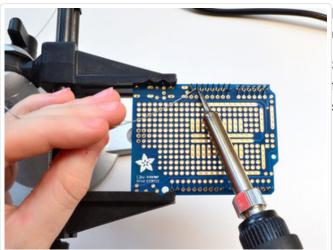
Now that you have aligned the stacky headers using an Arduino it's easy to finish the job
