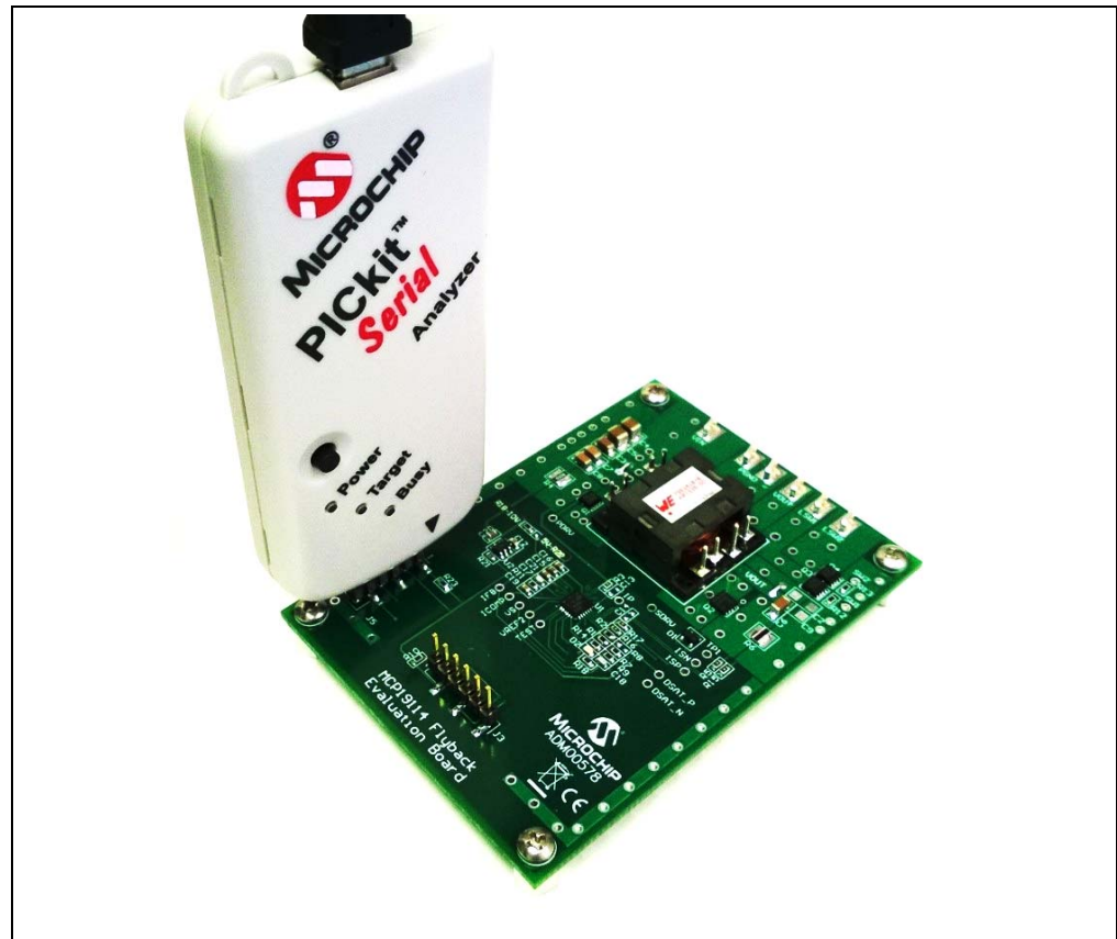
FIGURE 3-1: PICKit Serial Analyzer Connection to the Board.
