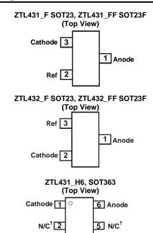
†Connected internally to substrate; should be left floating or connected to Anode
