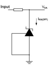
Figure 3. Test circuit for off state current
