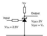
Single supply comparator with temperature compensated threshold
