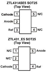
\*must be left floating or connected to pin 5
