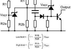
Over voltage / under voltage protection circuit
