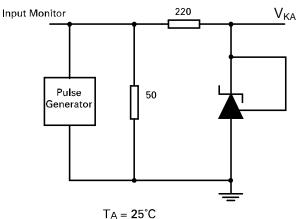
Test Circuit for Pulse Response
