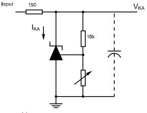
$V_{REF} < V_{KA} < 20, \ I_{KA} = 10mA, \ T_A = 25^\circ C$  Test Circuit for Stabilty Boundary Conditions
