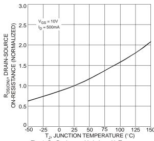
Fig. 4 On-Resistance Variation with Temperature
