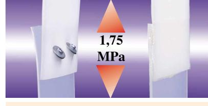
At 1,75 MPa, the overlapped plastic panels on the left elongated at the rivet. The overlapped panels bonded with 3M<sup>™</sup> Scotch-Weld<sup>™</sup> Adhesive DP-8005 on the right showed no visible signs of stress. Adhesive distributes stress more evenly eliminating the holes and stress points of mechanical fastening.
