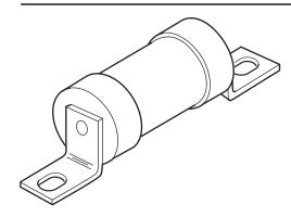
CATALOG SYMBOL: BAO INDUSTRIAL HRC FUSE OFFSET BOLTED TAGS PACKAGE QUANTITY: 20 80kA INTERRUPTING RATING MOUNTS IN CAMASTER CM63F SERIES OF HOLDERS
