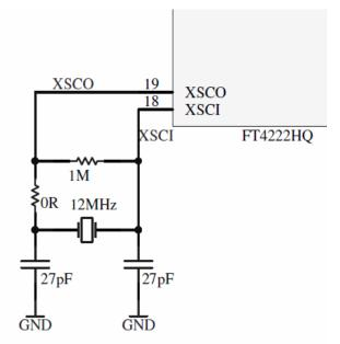
Figure 7.4 Recommended FT4222H Crystal Oscillator Configuration.
