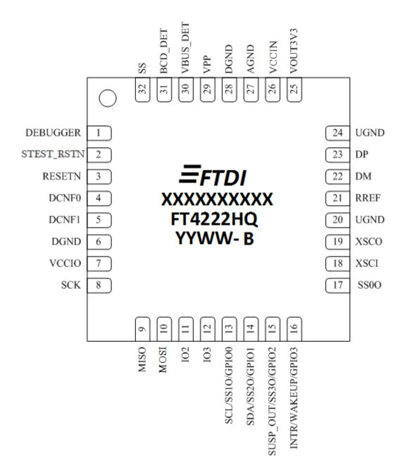
Figure 3.1 Pin Configuration VQFN-32 (top-down view)
