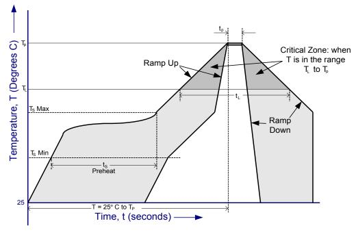
Figure 10.3 FT4222H Solder Reflow Profile
