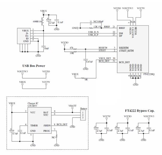
Figure 7.5 USB Battery Charging Detection
