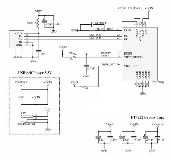
Figure 7.3 Self Powered Configuration with 3.3V Source Input
