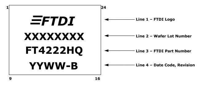
Figure 10.2 VQFN-32 Package Markings
