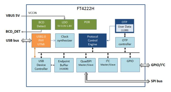
Figure 2.1 FT4222H Block Diagram
