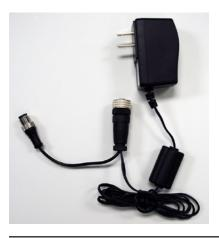
Part No: 14642 Model No: BWA-HW-026 Description: Splitter cable, wall plug for external power split to 5-pin Euro-style male and 5-pin Euro female (to power a M-H at 1 Watt while configuring it through the MHCT)
