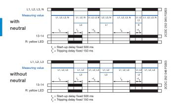
Function diagrams - Phase failure detection CM-PBE
