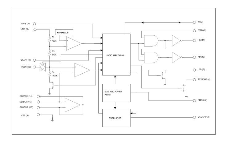
CMOS Ionization Smoke Detector ASIC with Interconnect, Timer Mode and Tone Select Product Specification
