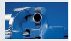
Jaws: Solid with drop forged body. Ground and CNC- machined for perfect grip. Induction hardened for endurance and added strength. Pipe jaws forged integral with the body, standard in all sizes. Ideal for plumbers and other professions where pipe and tube work is also part of the day.
