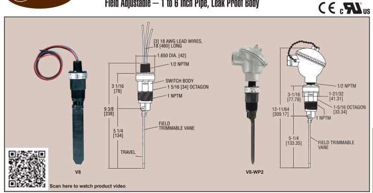
V8 Flotect<sup>®</sup> Flow Switch Protects Equipment: Operation is simple and dependable. In most applications, the switch is normally off while there is sufficient flow of liquid or air. When flow stops, the vane spring moves the vane, actuating a single pole double throw switch rated 5A @ 120/250 VAC to start or stop motor, pump, engine, etc. Operate a damper or valve; shut down a burner or actuate an alarm or signal, protecting unattended equipment from damage or loss of production.
