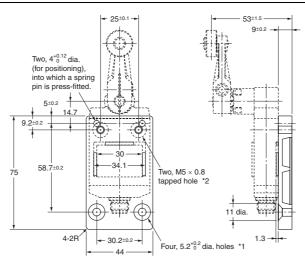
Note: Four hexagonal flat head bolts  $(M5 \times 0.8, length: 10)$ , two Allen-head bolts (M5  $\times$  0.8, length: 15), and two spring pins  $(4 \times 14)$  are included.
