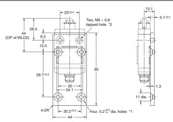
Note: Four hexagonal flat head bolts (M5  $\times$  0.8, length: 10) and two Allen-head bolts (M5  $\times$  0.8, length: 15) are included.
