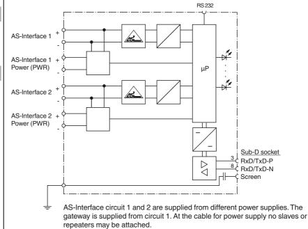
At the cable for AS-Interface circuit no power supplies or further masters may
