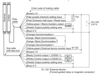
The diagram at left shows the configuration when using PNP output, interlock function "enabled (manual reset)" and external device monitoring function "enabled".
