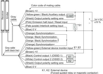
The diagram at left shows the configuration when using NPN output, interlock function "enabled (manual reset)" and external device monitoring function "enabled".
