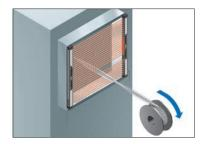
The floating blanking function allows you to disable up to three unspecified beams. Control output (OSSD) will not turn off as long as the number of interrupted beams is less than the set number of beams. This capability is convenient when an obstruction must move inside the detection area during setup changes or when loading materials inside the light curtain's detection area.
