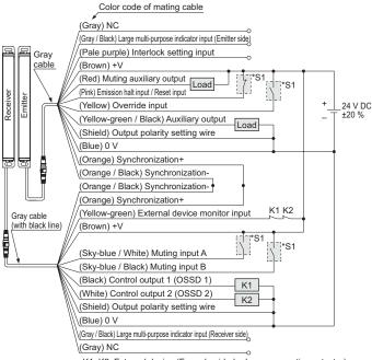
\*S1 K1, K2: External device (Forced guided relay or magnetic contactor)
