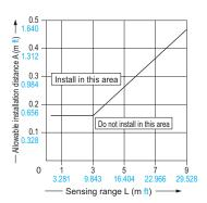
Note: The effective aperture angle for this device is ±2.5° or less (when L > 3m 9.843 ft) as required by IEC 61496-2, ANSI/UL 61496-2. However, install this device away from reflective surfaces considering an effective aperture angle of ±3° to take care of beam misalignment, etc. during installation.
