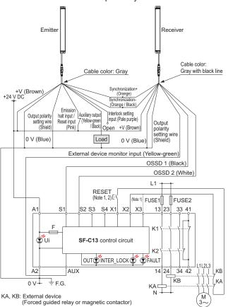
Notes: 1) The above diagram is when using manual reset. If automatic reset is used, disconnect the lead from X2 and connect it to X3. In this case, a reset (RESET) button is not needed.
