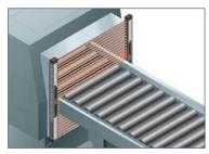
The **SFB-HC** handy-controller provides a fixed blanking function that prevents control output (OSSD) from turning off even if certain beams are interrupted. This capability is convenient in applications where an obstruction always interrupts certain beams. Additionally, a high level of safety is provided since control output (OSSD) is forcibly turned off in the event the obstruction moves outside the detection area.
