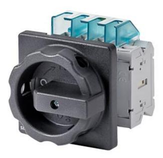
MAIN CONTROL SWITCH 3-POLE IU=25, P/AC-23A AT 400V=9,5KW 1NO+1 NC, FRONT MOUNTING FOUR-HOLE MOUNTING ROTARY ACTUATOR BLACK
