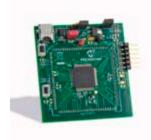
The PIC18F97J94 Demo Board/Plug-In Module (MA180034) is a board featuring the 100-pin PIC18FJ94 which supports the evaluation of 64-, 80-, and 100-pin devices within the PIC18F97J94 family of LCD/USB microcontrollers.
