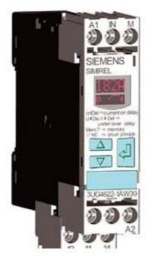
DIGITAL MONITORING RELAY CURRENT MONITORING, 22.5MM FROM 2 TO 500MA AC/DC OVERSHOOT A. UNDERSHOOT AC/DC 24 TO 240V DC AND AC 50 TO 60 HZ ON AND SPIKE DELAY 0.1 TO 20S HYSTERESIS 0.1 TO 250MA 1 CO CONTACT W. OR W/O ERROR MEMORY SCREW CONNECTION REPLACEMENT PRODUCT FOR 3UG3521-1AL20, 3UG3521-1AG20 AND 3UG3521-1AC48-0AA1
