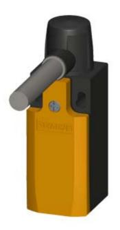
SIRIUS HINGED SWITCH PLASTIC HOUSING,31MM,EN50047 DEVICE CONNECTION 1X(M20X1.5) SNAP-ACTION CONTACTS 1NC/1NO INTEGR.,W. SOLID SHAFT D=10MM ACTUATING ANGLE 10 DEGR.
