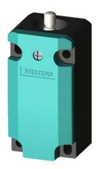
BASIC SWITCH FOR POSITION SWITCH 3SE5112, METAL ENCLOSURE, TO EN50041, 40 MM; 1X(M20X1.5) 1NO/2NC SLOW-ACTION CONTACTS WITH OVERLAP W/O ACTUATOR HEAD
