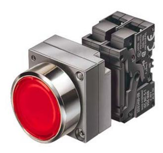
22MM METAL ROUND COMPLETE UNIT COMBINATION: ILLUMINATED PUSHBUTTON MOMENTARY CONTACT TYPE WITH FLAT BUTTON ILLUMINATED WITH INTEGRATED LED 24V AC/DC SCREW TERMINAL, 1NO WITH HOLDER WHITE
