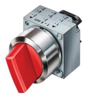
22MM METAL ROUND ACTUATOR: SELECTOR SWITCH LATCHING 3 SWITCH POSITIONS I-O-II NON-ILLUMINATED WITH HOLDER BLACK SOLVENT-RESISTANT NOT INSCRIBABLE WITH LASER
