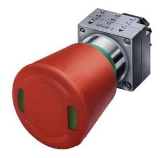
22MM METAL ROUND ACTUATOR: EMERGEN.-STOP MUSHR.PUSHB. 40MM LATCH.W. ROT.-TO-UNLATCH MECH. FRONT SWITCH POSITION INDICATOR WITH HOLDER RED
