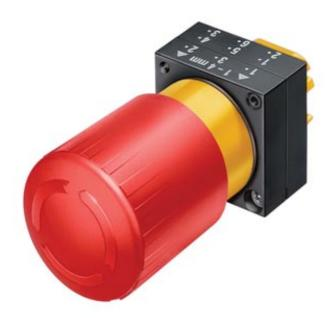
22MM PLASTIC ROUND ACTUATOR: EMERGEN.-STOP MUSHR.PUSHB. 32MM LATCH.W. ROT.-TO-UNLATCH MECH. WITH HOLDER RED
