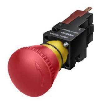
EMERGENCY-STOP MUSHROOM PUSHBUTTON, 16MM, ROUND, PLASTIC, RED, LATCHING, ROTATE-TO-UNLATCH MECHANISM, 1NC, WITH YELLOW BACKING PLATE, INSCRIPTION EMERGENCY-STOP
