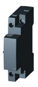
VOLTAGE RELEASE, AC 90...110V, 50/60HZ, 100% ED, AC 70...190V, 50/60HZ, 5SEC ED, DC 70...190V, 5SEC ED, W. SCREW CONNECTION; FOR CIRCUIT-BREAKERS, SZ S00/S0
